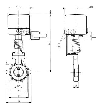
When installing the valve, allow the following minimum clearance from the wall or ceiling for mounting, connection, operation, maintenance etc.:
